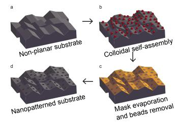
**Fig. 1** Conformal bottom-up nanopatterning of non-planar substrates. (a,b) Adsorption of colloids from aqueous solution onto a rough or micro-structured substrate of choice. (c) Etch mask deposition and beads removal. (d) Etch of the target substrate and removal of the mask.
