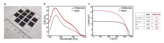
**Fig. 4** PolySi solar cells enhanced by conformal bottom-up nanopatterning (nominal bead size of 270 nm). (a) Photograph of the nanopatterned polySi cells (1 x 1 cm). The initial size of the nanopatterned polySi wafer before dicing (5 x 5 cm) is shown with dashed lines. (b,c) Electrical performances of a native polySi cell (black) and the best obtained nanopatterned polySi cell (red).
