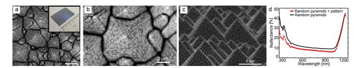
Fig. 5 Conformal bottom-up nanopatterning of pyramid-textured silicon substrates. (a,b) SEM images of pyramid-textured substrates with a metal etch mask. Inset in a: photograph of the nanopatterned substrate (5 x 5 cm). (c) Side view of a nanopatterned pyramid-textured substrate after dry etch and mask removal. (d) Reflectance of a pristine pyramid-textured surface (black) and a surface with added conformal nanopattern (red, nominal bead size of 270 nm).
