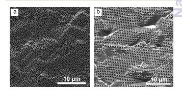
**Fig. 3** Comparison of polySi surface patterned by bottom-up nanopatterning (a) and nanoimprint lithography (b).
