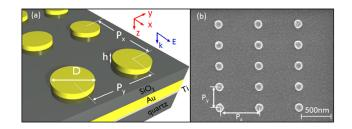
FIG. 1. (a) Schematic illustration of double-resonance gold nano-disk array substrate. (b) Scanning electron micrograph of a gold nano-disk array.
