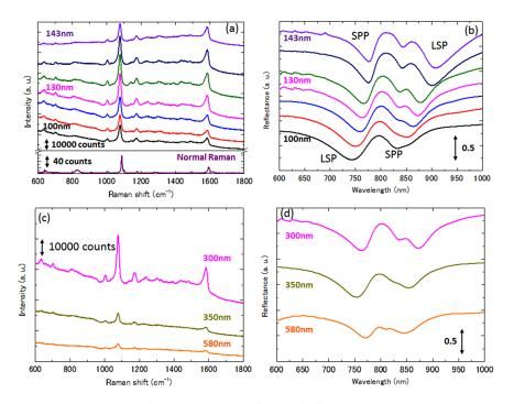
FIG. 4. (a) (Top panel) SERS spectra of 4-ATP on double-resonance nano-disk array substrates ( $P_x = 580$  nm and  $P_y = 300$  nm). For the spectra, the diameter changes from 100 to 143 nm. (Bottom panel) Normal Raman spectrum of 100  $\mu$ m thick 4-ATP film. (b) Reflectance spectra corresponding to (a). (c) SERS spectra as  $P_y$  changes from 300 nm to 580 nm ( $P_x = 580$  nm and diameter = 130 nm). (d) Reflectance spectra corresponding to (c).
