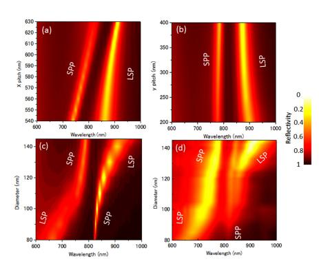
FIG. 2. Contour plots of calculated reflectance as functions of (a)  $P_x$  and wavelength ( $P_y = 300 \text{ nm}$ , diameter = 130 nm), (b)  $P_y$  and wavelength ( $P_x = 580 \text{ nm}$ , diameter = 130 nm), and (c) diameter and wavelength ( $P_x = 580 \text{ nm}$ ,  $P_y = 300 \text{ nm}$ ). (d) Contour plot of experimentally obtained reflectance as a function of diameter and wavelength ( $P_x = 580 \text{ nm}$  and  $P_y = 300 \text{ nm}$ ).
