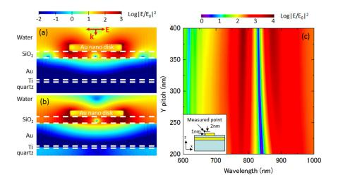
FIG. 3. Simulated electric field distributions for the structure with  $P_x = 580$  nm,  $P_y = 300$  nm, and d = 130 nm at (a) 785 nm (SPP resonance) and (b) 879 nm (LSP resonance). (c) Contour plot of electric field intensity as functions of  $P_y$ and wavelength ( $P_x = 580$  nm).
