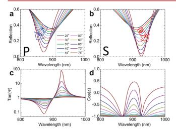
**Figure 3.** Angle-dependent simulation data for a periodic array of gold nanorings. (a,b) Simulated intensity based reflection spectra for P- and S-polarizations. (c) Simulated values of  $\tan(\Psi)$ , the reflection ratio between P- and S-polarizations. (d) Simulated values of  $\cos(\Delta)$  with  $\Delta$  the phase difference between both polarization states.
