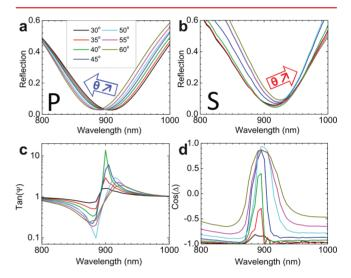
Figure 2. Angle dependent measurement data for gold nanorings. (a,b) Measured intensity based reflection spectra for P- and Spolarizations. (c) Measured values of  $\tan(\Psi)$ , the amplitude reflection ratio between P- and S-polarizations. (d) Measured values of  $\cos(\Delta)$ , with  $\Delta$  the phase difference between both polarization states.
