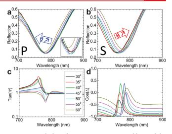
Figure 4. Angle-dependent measurements on gold nanodisks. Reflection spectra for P- (a) and S-polarization (b). (c) Reflection ratio  $tan(\Psi)$ . (d) Phase difference  $cos(\Delta)$ .
