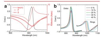
Figure 5. Refractive index sensing measurements on gold nanodisks and nanorings for  $45^{\circ}$  incidence. (a) Comparison of phase-sensitive measurements (black) and intensity based measurements (red) on gold nanorings in air, illustrating a dramatic line width reduction in the phase-difference between P and S. (b) Refractive index sensing measurements on disks and disks with variable concentrations of glycerol in water.
