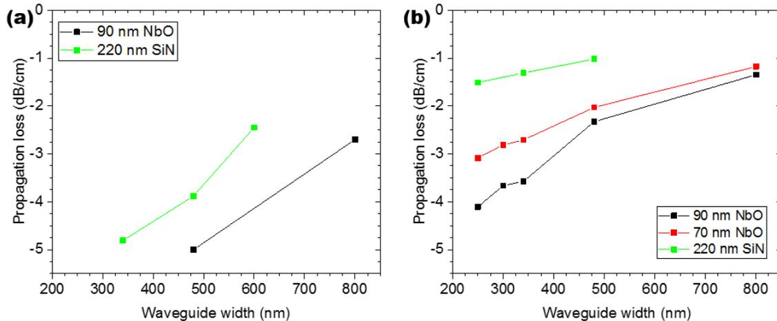
Figure 2: Waveguide losses at 638 nm wavelength before (a) and after (b) top cladding deposition for different NbO strip waveguides and SiN as a reference platform.
