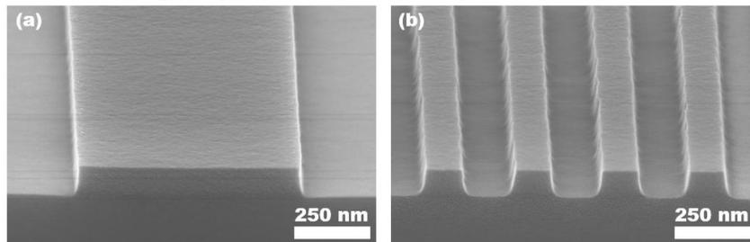
Figure 1: Scanning electron microscope images of the patterned NbO waveguides (a) and grating couplers (b) after lithography and etch.
